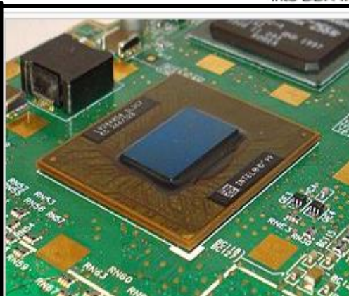
Intel Mobile Celeron in a BGA2 package (FCBGA-479); the die is blue
